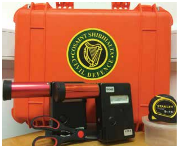
Graetz meters used to take background radiation readings.
