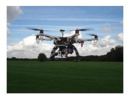
The second unit is a DJI S800 EVO with a Sony NEX7 (High Spec) camera, mounted on a three axis stabilised gimbal. This system again provides high quality imagery of the surveyed ground area to the receiver screens on the ground.
